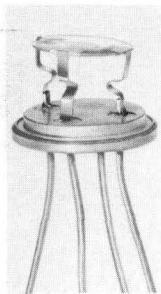
Fig. 5. Close-up view of quartz sensor mounted on header. Sensor is later sealed in helium atmosphere.
