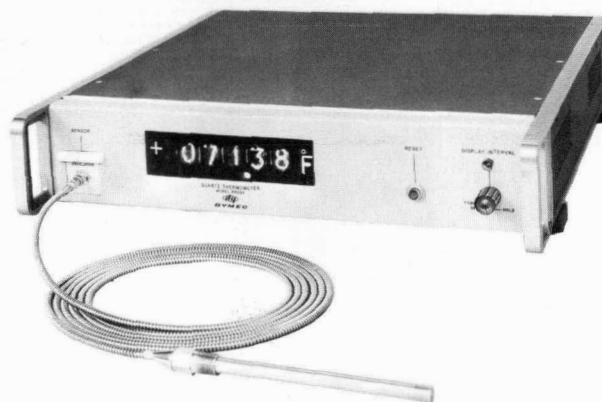
Fig. 7. Single-channel Thermometer. Sensor oscillator can also be used externally for remote measurements.
